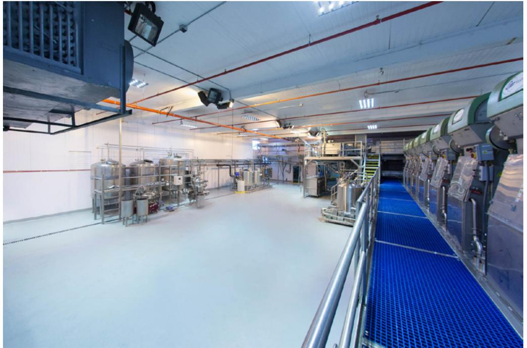
the contractor surface-prepped the entire cooler floor by grinding and shot-blasting, preparing it for the contoured floor that required up to 3-inches of epoxy mortar. Crews sloped the final surface from the outside walls to new trench drains.
